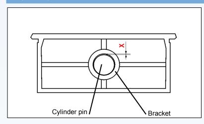
Check the space "X" between the bush and the cylinder pin using a feeler gauge. In case this exceeds 1.5mm the pin or bush may have worn out and extra attention is required.
